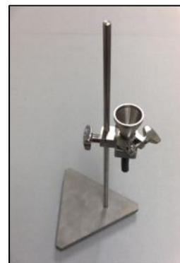
Figure 4: IMD-A 350 isokinetic probe with stand
