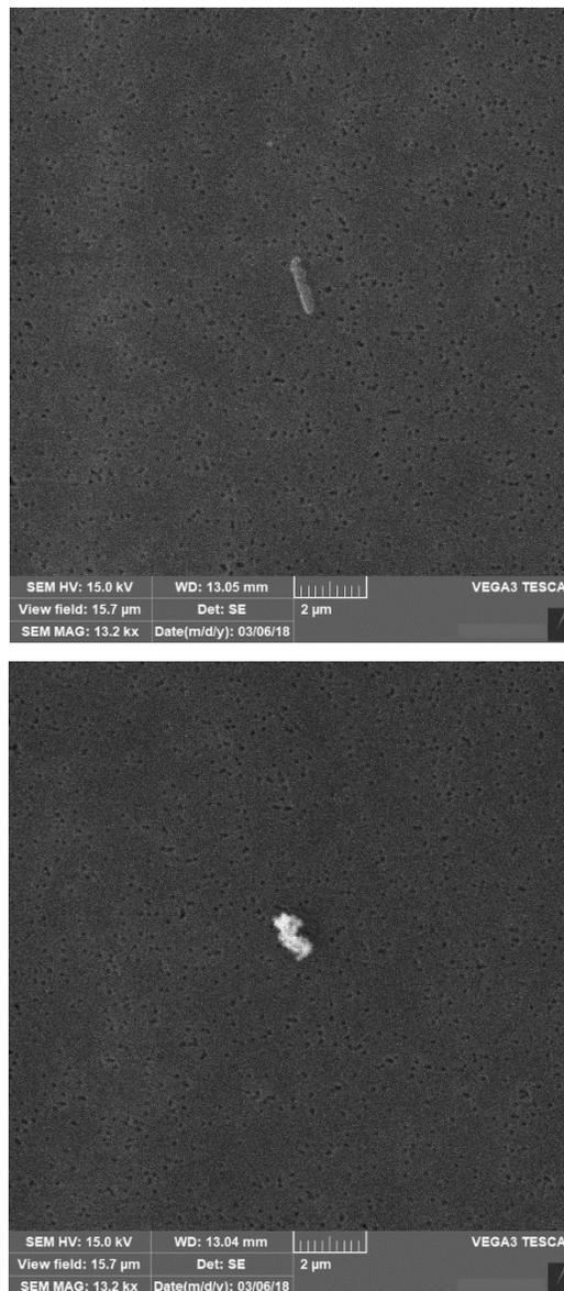
**Figure 1:** SEM images of two particulate in the water sample. The rod-shaped particle on the top is identified as a bacteria (i.e. biologic particle) and the particle on the bottom as a rouge particle.
