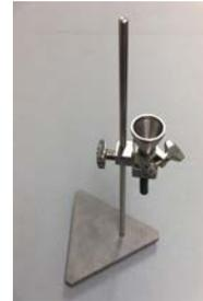
Figure 1: IMD-A 350 isokinetic probe with stand
