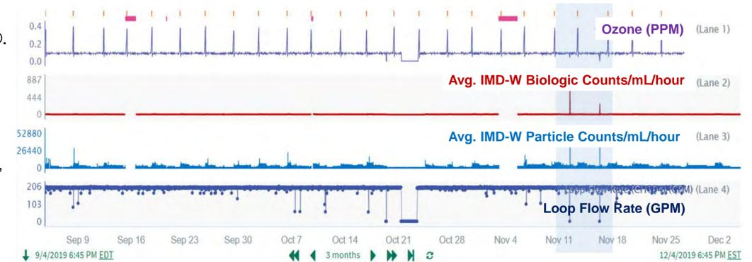
Loop process data streams can be compared to investigate root cause of a spike in particle and biologic counts observed (blue shaded rectangle).
