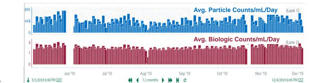
Based on significant IMD-W continuous data since May of 2019 showing general stability in counts and ability to continuously monitor counts after a change, plan to investigate reduction in ozone sanitization frequency, cycle time or concentration to support energy reduction.
